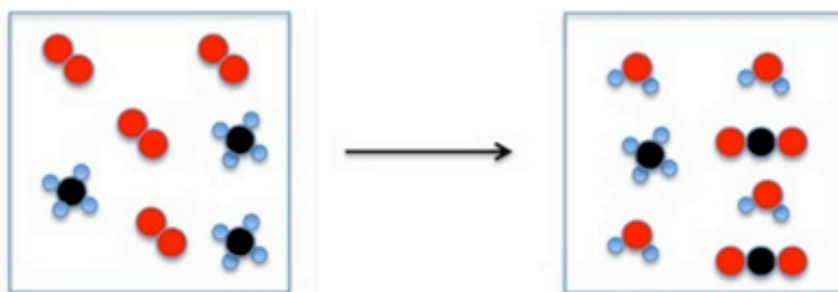
Figure 1. A particulate nature of matter (PNOM) diagram representing the complete combustion of three moles of methane in the presence of four moles of oxygen. In this diagram, each black sphere represents a carbon atom, red spheres represent oxygen atoms, and small light blue spheres represent hydrogen atoms.
